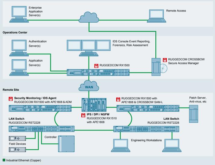
RUGGEDCOM CROSSBOW is a secure access management solution designed to provide cyber security compliance including NERC CIP access to Intelligent Electronic Devices (IEDs).
